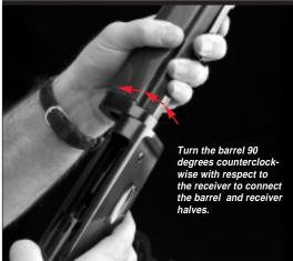
6. With the barrel extension inserted, turn the barrel counterclockwise 90° to tighten the connection (see Figure 9). Very little force should be required to turn the barrel assembly into its proper position.
